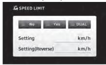
This function limits the maximum vehicle speed to the setting speed; and forward/backward speeds are identical in the case of regular setting, whereas forward/backward speeds differ in the case of dual setting.
