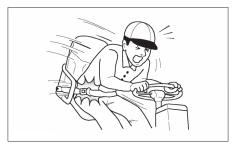
In the event of tip over, the seat and restraint system should be inspected for damage and replaced, if necessary.
