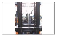
Inspect the part of the chain that is normally operated over the crosshead roller. When the chain bends over the roller, the movements of the parts against each other causes wear.
