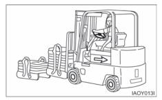
Use special care when operating on grades. Do not angle across or turn on grades. Do not use a lift truck on slippery grades. Travel with forks downgrade when unloaded. Travel with load upgrade.
