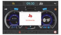
Display that notifies the operator of automatic DPF regeneration / SCR cleaning
