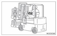
Tilt an elevated load forward only when directly over unloading area and with load as low as possible.
