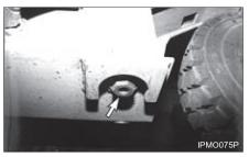
Remove the hydraulic tank drain plug located on the bottom of the frame. Allow the oil to drain in a suitable container. Clean and install the plug.
