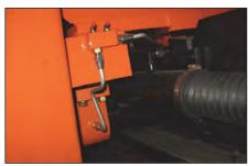
Apply lubricant to the fitting at the end of the tube connected to the steering axle support. Lubricate the point in the event of abnormal noise.
