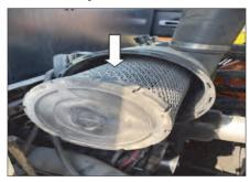
Remove the secondary element. Inspect the gasket between the air cleaner housing and the engine inlet. Replace the gasket if it is damaged.
