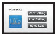
This option enables the operator to measure and limit the weight of the load using the LCD display. Use "WEIGHT SCALE" under the "VEHICLE" menu.
